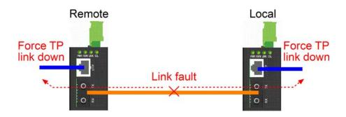
The following figure illustrates another example. A link fault happened on the copper cable is detected by the remote end. The fault is forwarded to the fiber segment and also forwarded to the copper cable at the local end by remote device and local device respectively.
