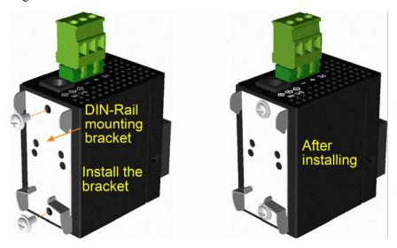
2. Attach bracket to the lower edge of the DIN rail and push the unit upward a little bit until the bracket can clamp on the upper edge of the DIN rail.
