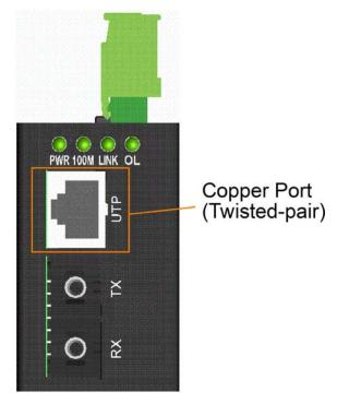
The copper port is featured to support connection to:
