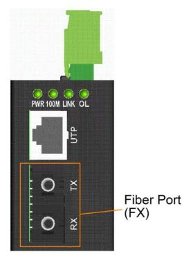
The fiber port operates on 100Mbps and full duplex. A variety of fiber options is provided as follows:
